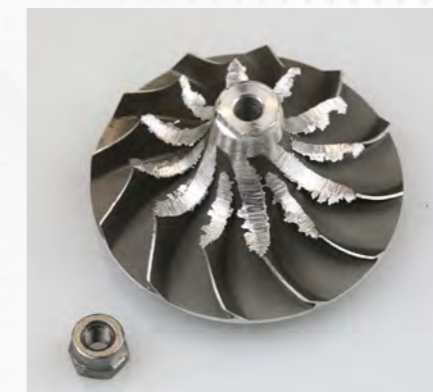
damage to compressor wheel blade due to loose nut
