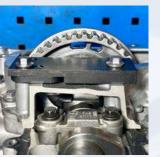
Exhaust Camshaft Locking Tool - 1.2 GDi PureTech EB2 - Euro 6.3 / 6.4 - Citroën - Peugeot - DS -Opel/Vauxhall
