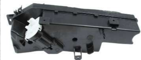
PEF Additive Reservoir Part No: 584-0012 Application: PSA Berlingo & Partner 2011 > 2016
