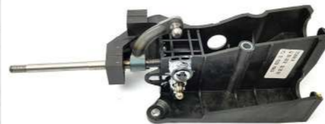
Gear Lever / Linkage Part No: 414-0015 Application: PSA Nemo & Bipper. Fiat Fiorino, Qubo
